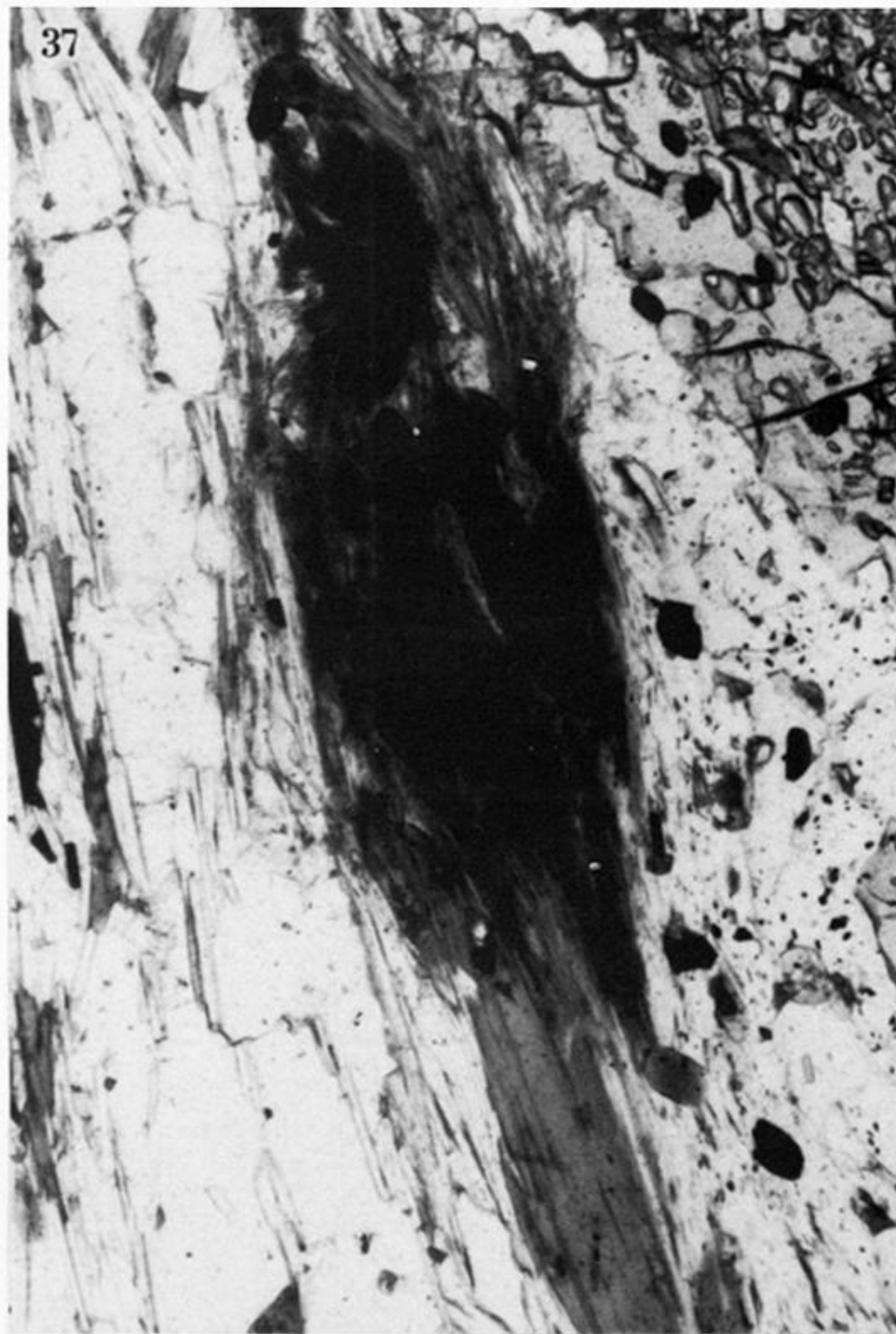
FIGURE 37. Enlargement of grain 1 of figure 36, showing clear biotite at centre right of photograph of figure 36 merging into turbid dark material towards centre of photograph. Wispy sillimanite has developed round the margins of the dark material, particularly towards the top of the photograph. Transmitted plane polarized light. (Magn. \times 50 .)
