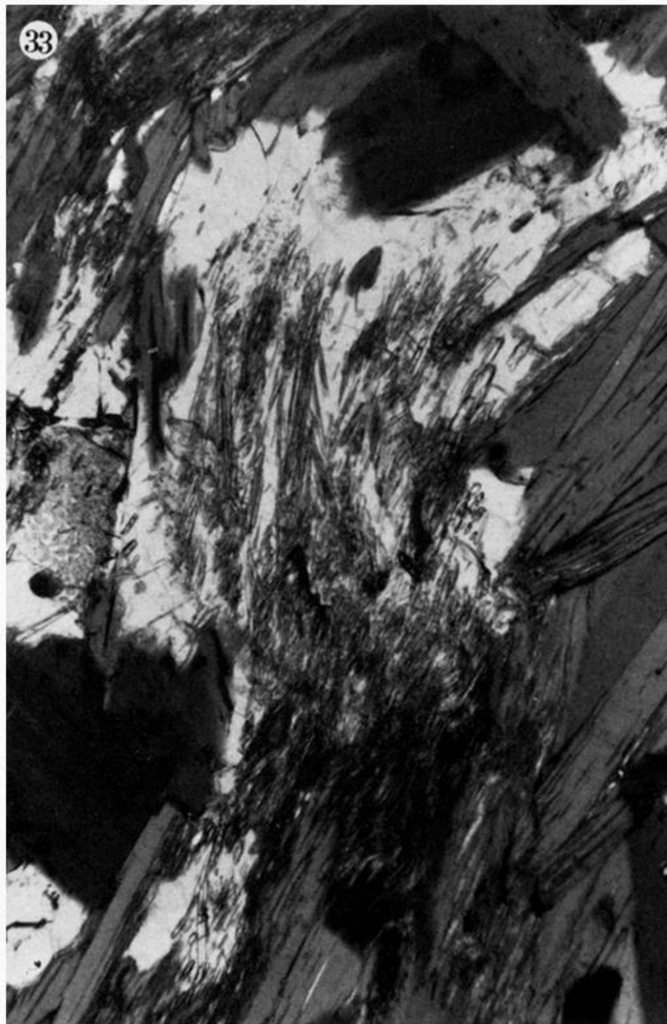
FIGURE 33. Enlargement of sudoitic chlorite of lower right of figure 31 (see lower arrow of figure 31) showing mode of occurrence of sillimanite in sudoitic chlorite analogous to that in cordierite, and analogous relations with unaltered biotite. Transmitted ordinary light. (Magn. \times 96 .)
