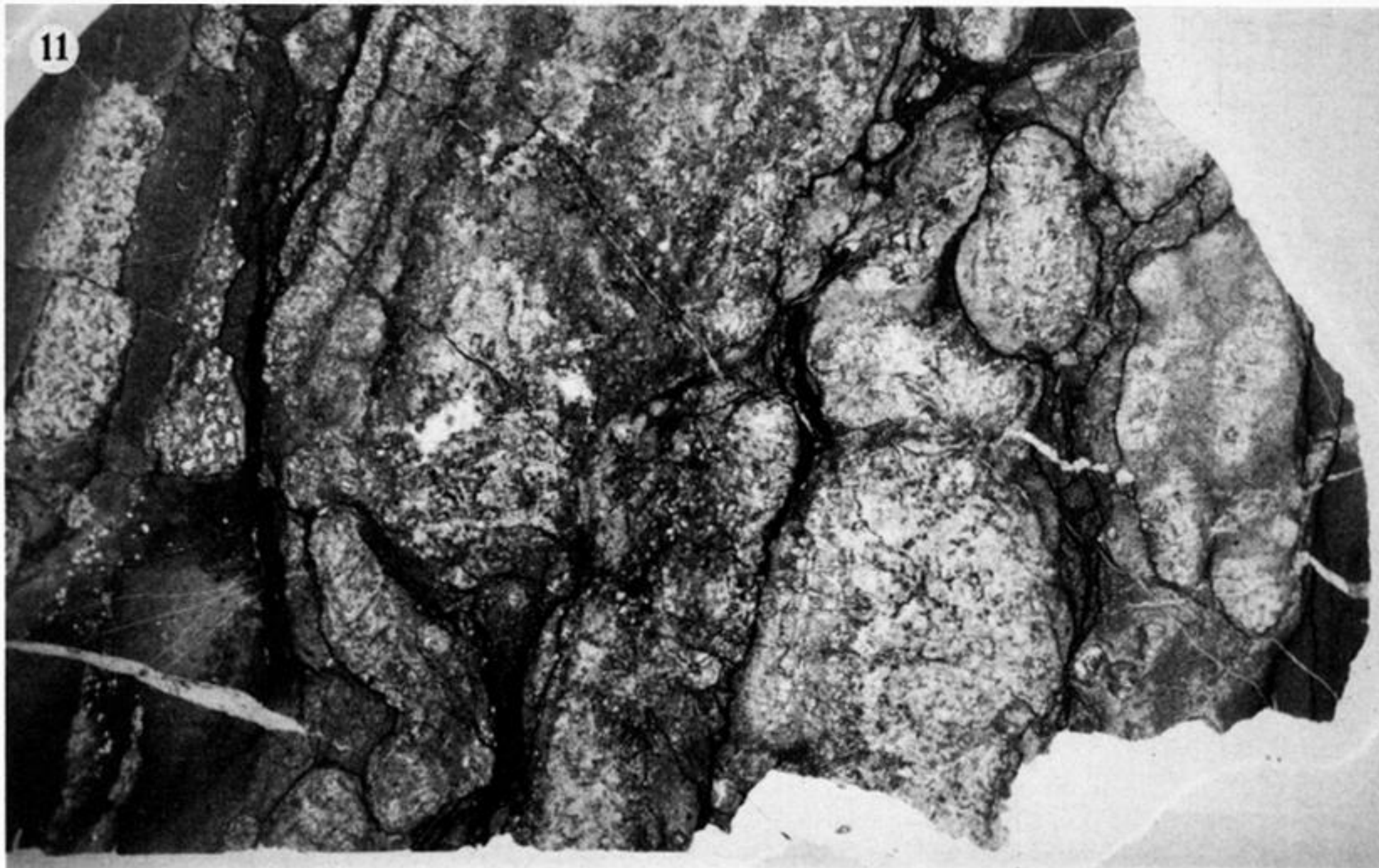
FIGURE 11. Calc-silicate and associated unmetamorphosed carbonaceous shaley-silty sediment in core from the Brindabella stratiform zinc sulphide bearing occurrence, southern New South Wales. The calc-silicate consists of what appear to be composite concretions of grandite garnet (light grey) and epidote (slightly darker grey). Ordinary light. (Magn. \times 5 .)
